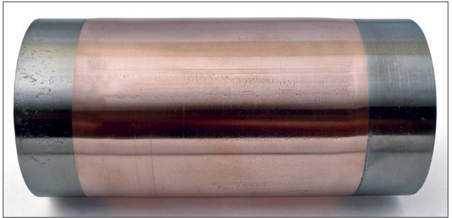
Fig. 3 — Two different metals joined by FRW.
