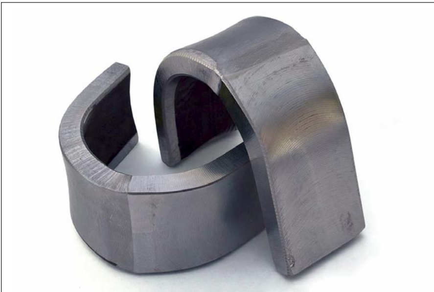
Fig. 2 — A full-strength weld created with the FRW process.
