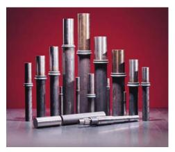
exceeded. Close state of the art control via monitoring and visual graphing during the weld process and post weld ultrasonic inspection procedures ensure consistent weld joint integrity through a very robust process. Production controls monitor RPM, axial load and displacement of material during welding.
